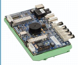
The GTSYNC Synchronization Card is used to synchronize the simulation time step to an external time reference (e.g. GPS clock) in order to eliminate this undesirable drift. The GTSYNC connects to a GT port on the back of the GTWIF card.
