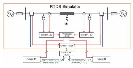
The RTDS Simulator's IEC 61850 communication capability is provided by the GTNETx2 card with the Sampled Values (GTNET-SV) and/or GOOSE (GTNET-GSE) firmwares installed.
