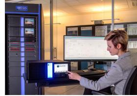
system. As simulation parameters are modified and contingencies are applied, the user can watch the power system respond in real time.
