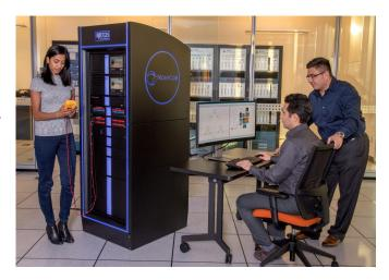
multicore processor housed in units called chassis that allow easy expansion of the Simulator's computing capability as required. Using the RTDS Simulator, analytical studies can be performed much faster than with offline EMT simulation programs.
