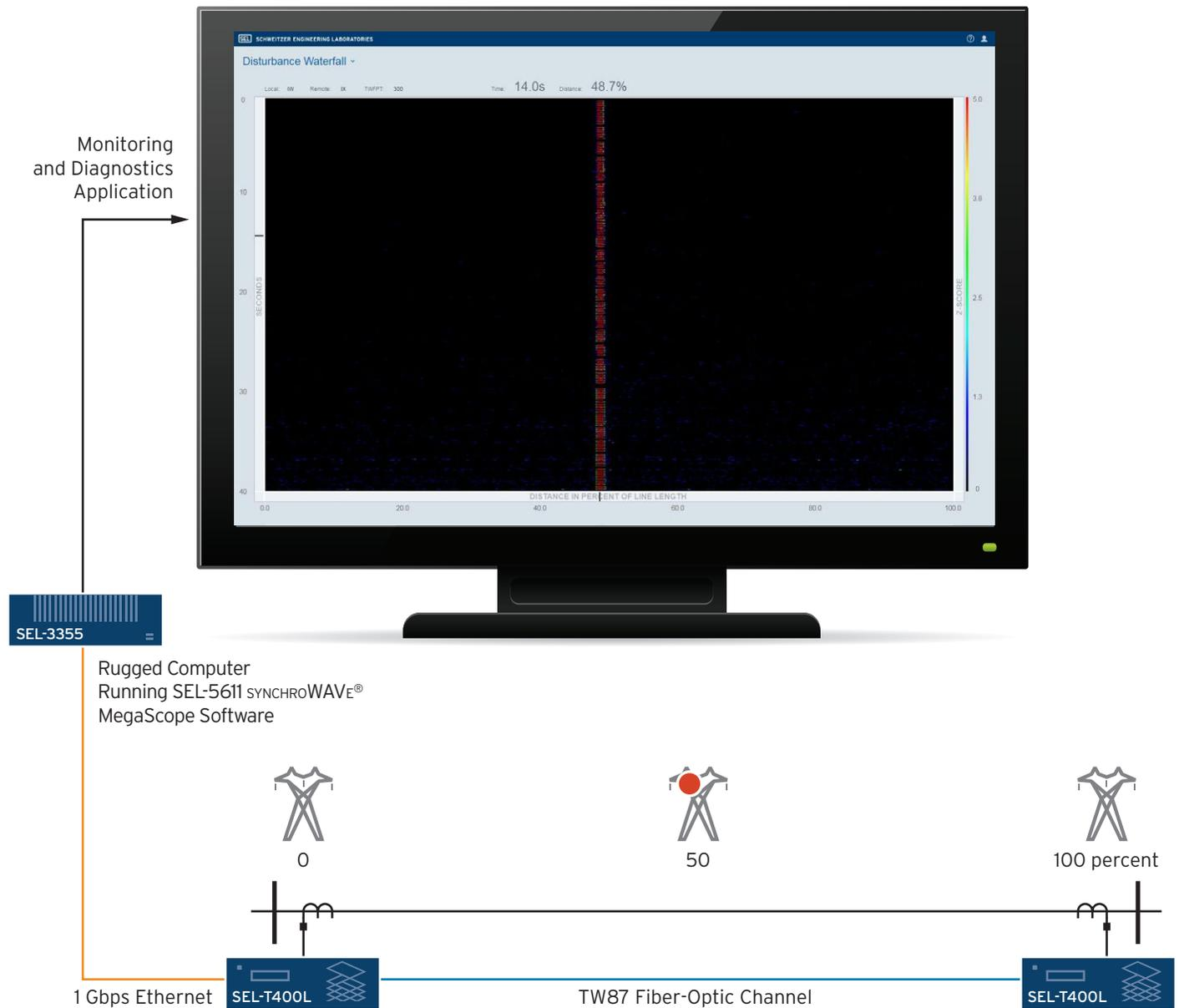
You can correlate local and remote current traveling waves using the SEL-T400L megahertz data. The red mark indicates the location and timing of a high-frequency persistent event, such as a failing insulator.
