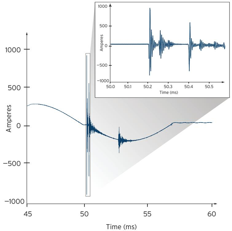
High-resolution oscillography shows a breaker restrike while de-energizing a shunt reactor.
